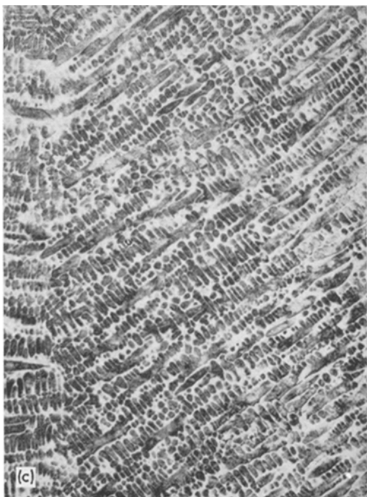
Figure 2 Variation of microstructure with cooling rate for Maraging 300 alloy. (a) Gas quench, (b) liquid quench, (c) chill cast. \times 188 .
